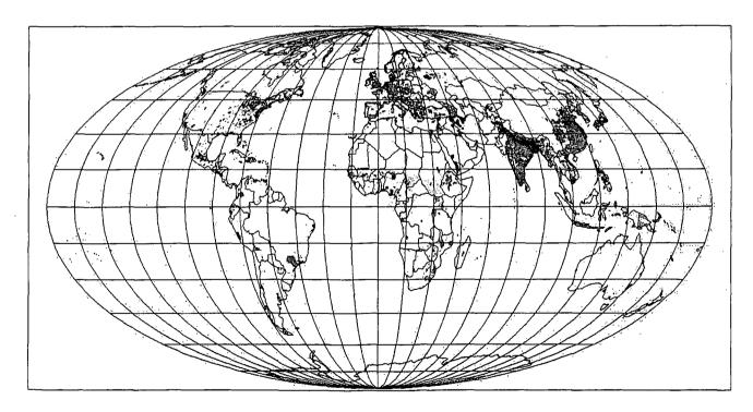
Figure 5.62. Annual average local deficit of the supplies of electricity and biofuels (such as biogas or hydrogen) relative to demand (all demand except food and transportation) on an area basis, according to the centralised 2050 scenario. (average demand minus supply in W/m² is shown if positive; scale given in Figure 5.28b).
