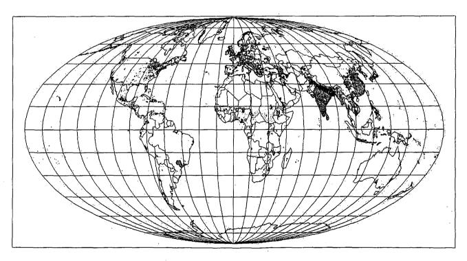
Figure 5.60. October local deficit of the supplies of electricity and biofuels (such as biogas or hydrogen) relative to demand (all demand except food and transportation) on an area basis, according to the centralised 2050 scenario. (average demand minus supply in W/m<sup>2</sup> is shown if positive; scale given in Figure 5.28b).
