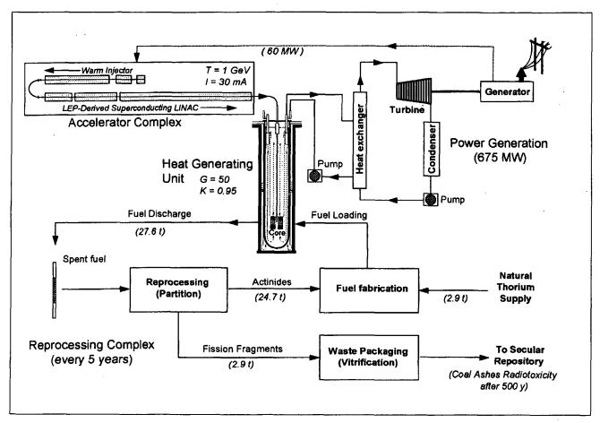
Figure 4.2. The energy amplifier fuel chain concept. The fraction of the generated electricity that has to be used for powering the accelerator is indicated. The reprocessing step is essential for the resource viability of the system (Rubbia and Rubio, 1996).
