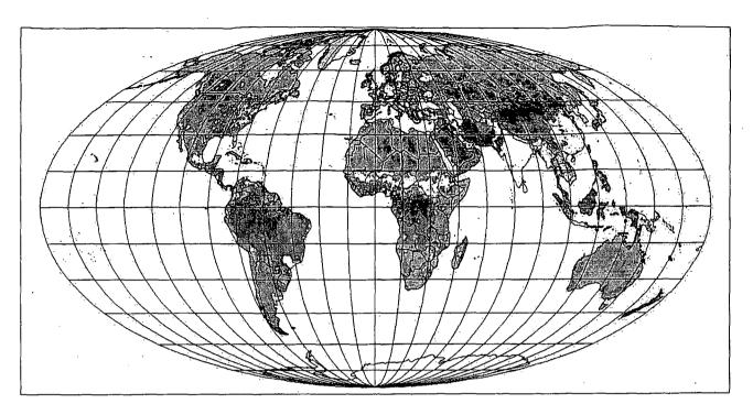
Figure 5.59. October local surplus of supplies of electricity and biofuels (such as biogas or hydrogen) over demand (all demand except food and transportation) on an area basis, according to the centralised 2050 scenario. (average supply minus demand in W/m<sup>2</sup> is shown if positive; scale given in Figure 5.11d).
