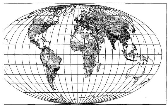
1. Total energy that must be delivered to the end-users in the 2050 energy demand scenario (including direct delivery of fuels and electricity, environmental heat and food energy), expressed as W/m<sup>2</sup> of land area. The scale is given in Fig. E.1a.
