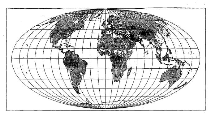
Figure 5.61. Annual average local surplus of supplies of electricity and biofuels (such as biogas or hydrogen) over demand (all demand except food and transportation) on an area basis, according to the centralised 2050 scenario. (average supply minus demand in W/m<sup>2</sup> is shown if positive; scale given in Figure 5.11d).
